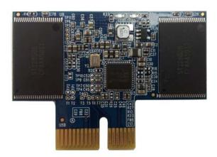
Super Talent's new compact PCle Flash Disk Module may be small in volume-but is no slouch when it comes to read/write performance even conditions deemed too harsh for hard disk drives. Unlike out dated hard drives, this PCle SSD holds the ability to provide sufficient storage space and enhanced boot times on your O/S-all the while insuring the ability to perform under vibration, and volatile temperatures.
