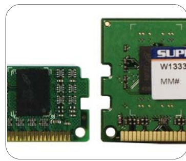
VLP memory (left) vs. standard memory (right)
