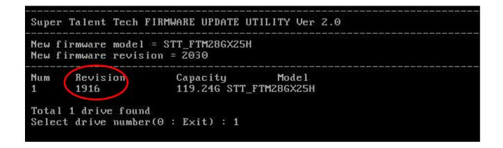
3). Type the drive number '1', and press <Enter>. The new F/W 1916 is loaded into the drive.
