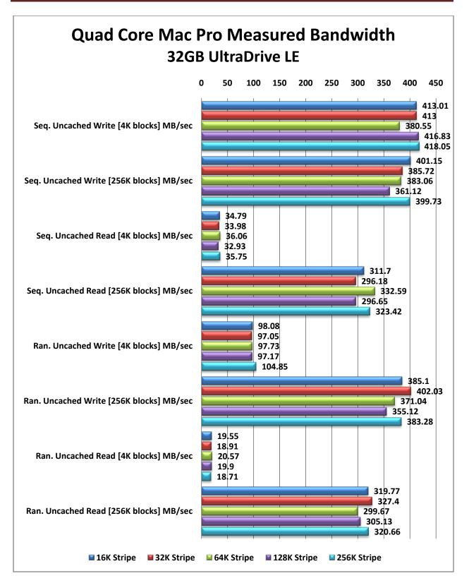
Figure 11: Mac Pro 32GB UltraDrive LE Stripe Test Measured Bandwidth
