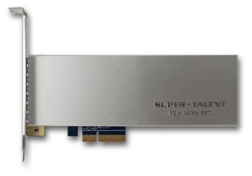
SuperCache is a PCIe NVMe Add In Card type Solid State Drive. It supports a max read speed of up to 3.0 GB/sec and a max write speed as fast as 2.2 GB/sec for Audio/Video Cache application. It also has a great performance of Random 4KB Read/Write up to 360K/500K IOPS. This AIC can also fit into 1U/2U/4U Rack Server System.
