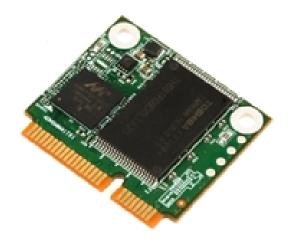
The mSATA mini SJ2 provides valuable embedded storage in a mSATA form factor. With read speeds up to 300MB/s and write speeds up to 100MB/s, the mini SJ2 delivers fast and reliable performance. This product has a SATA III interface and is available in capacities of 16, 32, and 64GB. The mSATA mini SJ2 is ideal for use in mobile and tablet technologies.
