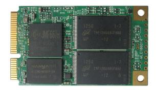
The mSATA DX1 provides high speed and reliable performance with speeds of up to 480MB/s read and 300MB/s write. The DX1 comes in a mini PCle form factor with a SATA III interface. This device is available in both MLC and SLC NAND flash. The DX1 comes in capacities of 32, 64, 128 and 256GB. The mSATA DX1 is perfect for mobile and tablet technologies.
