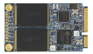
The CoreStore Plus is an ultra-small form factor SSD designed to fit into a standard Mini-PCIe slot. This mini-PCIe card form factor is perfect for embedded applications, netbooks, notebooks, and tablets where hardware space is limited.
