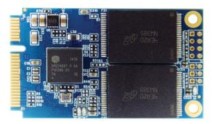
mSATA SJ2 features outstanding performance. Available in 16GB to 128GB capacities, this drive complies with the SATA-II/SATA-III standards and provides read speeds of up to 480 MB/s and write speeds of up to 160 MB/s. The mSATA SJ2 is perfect for mobile and tablet technologies to increase performance for all applications.
