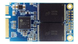
mSATA SJ4 features outstanding performance. Available 128GB to 1TB capacities, this drive complies with the SATA-II/SATA-III standards and provides read speeds of up to 520 MB/s and write speeds of up to 460 MB/s. The mSATA SJ4 is perfect for mobile and tablet technologies to increase performance for all applications.
