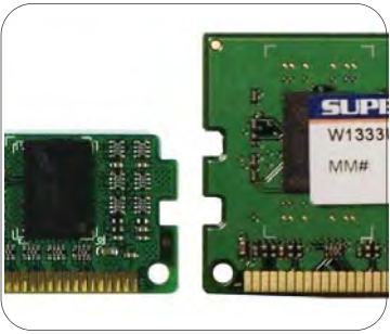
VLP memory (left) vs. standard memory (right)
