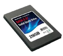
A Solid State Disk (SSD) is a storage device that is based on semiconductors rather than rotating magnetic platters. Most SSDs, including Super Talent's offerings, are based on NAND Flash chips because they are fast, highly reliable, widely available and are non-volatile.
