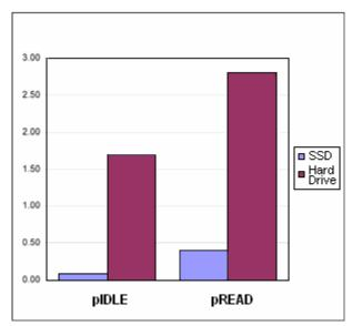
Figure 1: Typical Power Consumption in Watts
