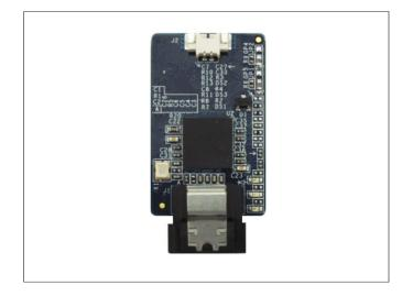
If space is a limiting factor, Super Talent has a sleeker disk on module (DOM) design available for netbooks, small form factor computers, and embedded systems. Despite its small size, this flash based product takes advantage of multi-level cell (MLC) technology. The standard 7-pin SATA connection ensures speed performance while the built in error correcting code (ECC) and error detection and correction (EDC) protect the data's integrity.
