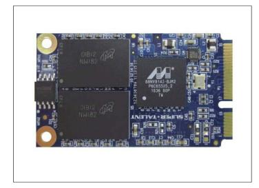
The CoreStore MV is an ultra small form factor SSD designed to fit in to a standard Mini-PCIe (30x50.95mm) slot. Featuring the new Marvell controller (88NV9143), latest ONFi 2 flash, the CoreStore MV offers huge performance and an ultra-compact size. The standard mini-PCIe card form factor is perfect for Embedded Applications, Netbooks, Notebooks and Tablets.
