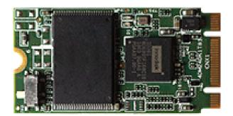
The M.2 SATA ST4 is substantially smaller, lighter and consumes less power compared to hard drives, yet has sufficient storage space to load an O/S and serve as a bootable drive for embedded applications. Moreover, these devices have excellent resistance to shock, vibration, dust, temperature extremes and other environmental hazards. M.2 SATA ST4 features outstanding performance and is available in 128GB to 1TB capacities.
