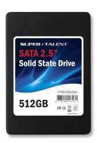
The DuraDrive AT is a solid state drive that provides high reliability and performance for industrial applications. The AT has excellent resistance to shock, vibration, dust, temperature extremes and other environmental hazards. It is built with the standard 2.5-inch form factor and a SATA-III interface. This drive is geared specifically for applications that require high shock and vibration tolerance.
