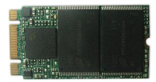
The NGFF ST1 is a NAND flash memory device which provides high reliability and high performance for storage media. NGFF ST1 is substantially smaller, lighter, and consumes less power while still providing sufficient storage space to load an OS and serve as a bootable drive for embedded applications.
